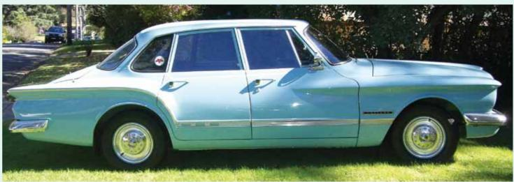
**The "S" Series** is very similar in appearance to the "R" Series with outward cosmetic changes distinguishing it from its predecessor. Removed was the fake wheel mold on the boot lid, the "cat's eyes" tail lights were changed to a more conventional tail light assembly, a different grille installed and changes to much of the chrome work. The floor mounted manual shift was moved to the steering column plus several other mechanical alterations were included.
